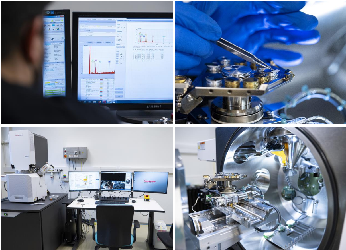
Fig. 3. Morphological analysis of thin films and coatings using Scanning electron microscopy.
